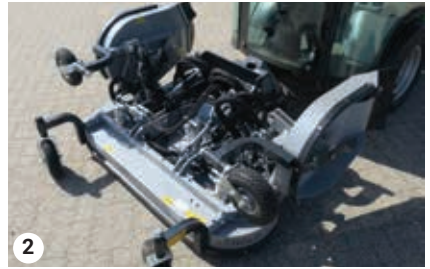
Blades in lifted wings will automatically stop
